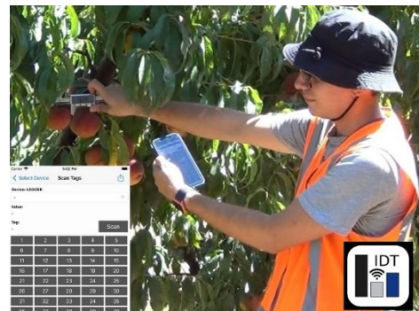
Picture 7: Digital Bluetooth callipers with DataLogger smartphone app for fruit size
