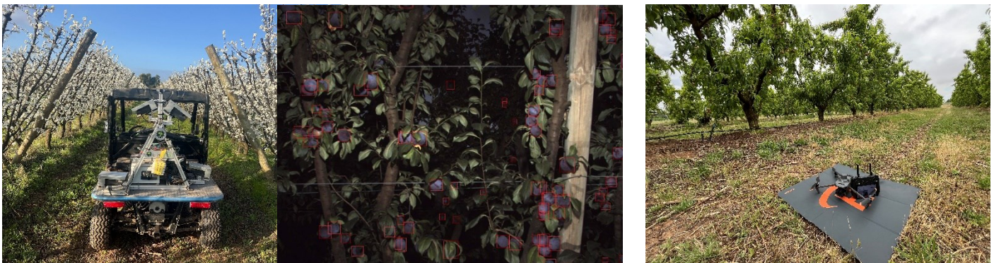
Picture 2: Green Atlas Cartographer to scan blossom load (left) & an example high resolution image of a plum tree detecting fruit size (red boxes) and fruit number (right).
