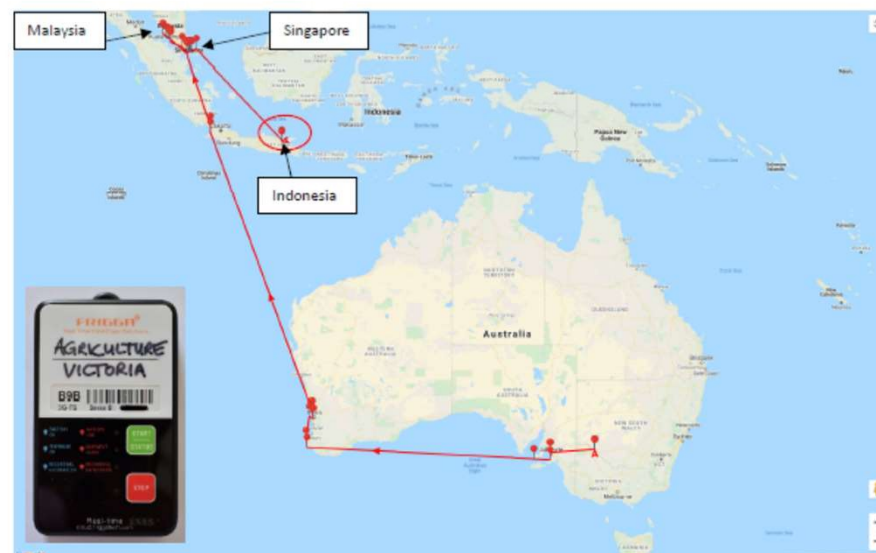
Figure 1. A real-time temperature logger (inset) used to monitor a sea freight consignment of 'Crimson Seedless' table grapes from Australia to Indonesia. Map is a screen shot of the vessels route, which was taken from a dashboard developed by DAF, Queensland. Photo courtesy of Glenn Hale.
