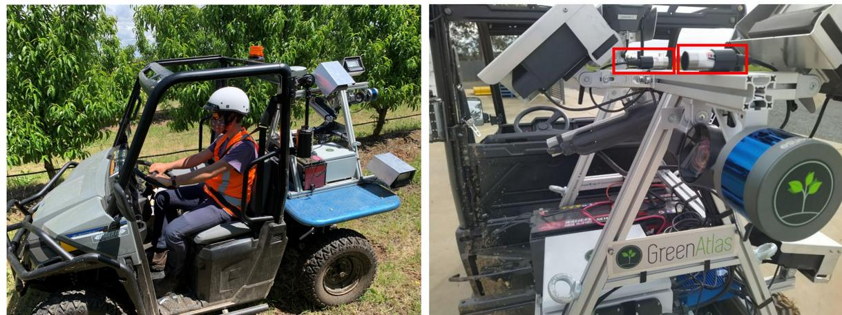
**Figure 1** Ground-based platform (Green Atlas Cartographer) equipped with Enviro-Therm™ infrared sensors (Everest Interscience).
