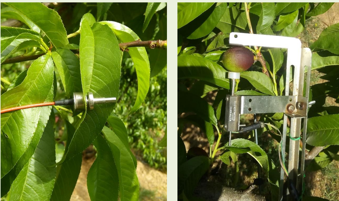
Figure 2. LPCP probe (left) and fruit gauge (right) on a 'September Bright' nectarine tree at stage I.
