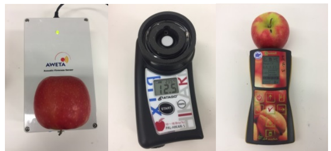
Figure 1. Three non-destructive instruments for measuring apple quality; AWETA for acoustic firmness (left), a PAL - Infra-red refractometer for soluble solids concentration (centre) and DA-meter for fruit maturity (right). Photos: Glenn Hale.
