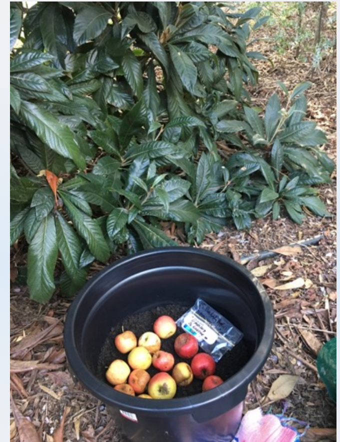
Field emergence chamber (uncovered) with potting mix, infested Pink Lady apples and digital temperature logger in place on-site in a Cobram backyard beneath a loquat tree.
