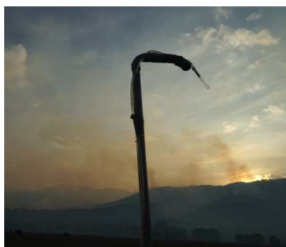
Figure 3. A Tenax tube attached to a nephelometer inlet tube enabling smoke taint compounds to be determined from controlled burns or bushfires.
