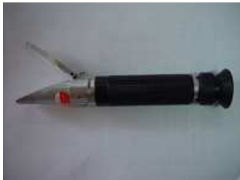
Figure 2: Hand held refractometer used to test TSS
