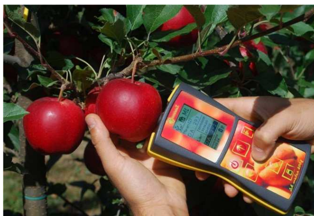
Figure 3: DA meter recording maturity in apples.
