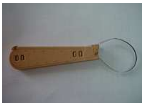
Figure 4: A Cranston gauge used to measure fruit size
