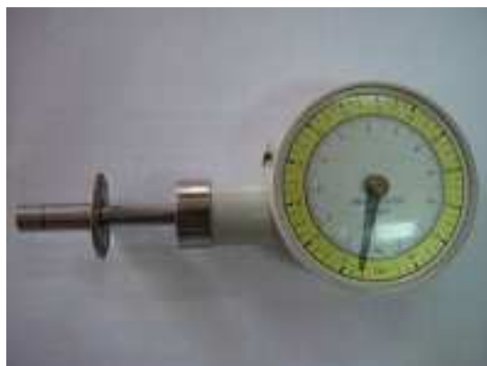
Figure 1: Penetrometer with an 8mm head used to test flesh firmness
